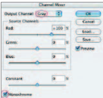
FIGURE 4-14. CHANNEL MIXER. Selecting Monochrome converts the image to black and white with default settings that derive input only from the red channel.
